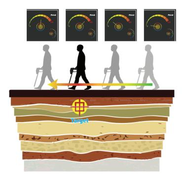
After performing the balance operation, move over the scan area while maintaining an equal distance between the tip of the device and the ground.
